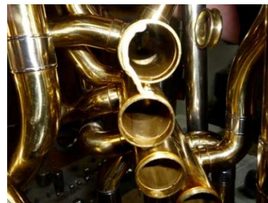
A tuba valve with a foreign substance oozing out. Before cleaning.
