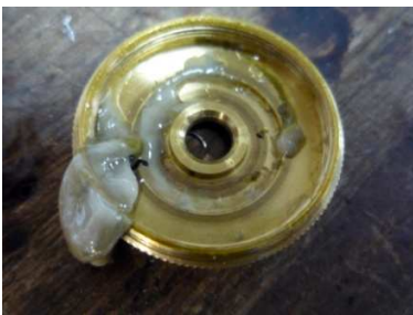
A tuba valve cap with a foreign substance oozing out of the valve cap. Before cleaning.
